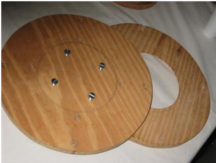
He showed us a clamp for bowls for those who do not have a vacuum chuck.
