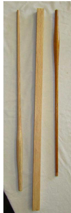
John Crede turned "impossible" spindles for a contractor using his metal lathe and his woodturning lathe. Nice work, John.
