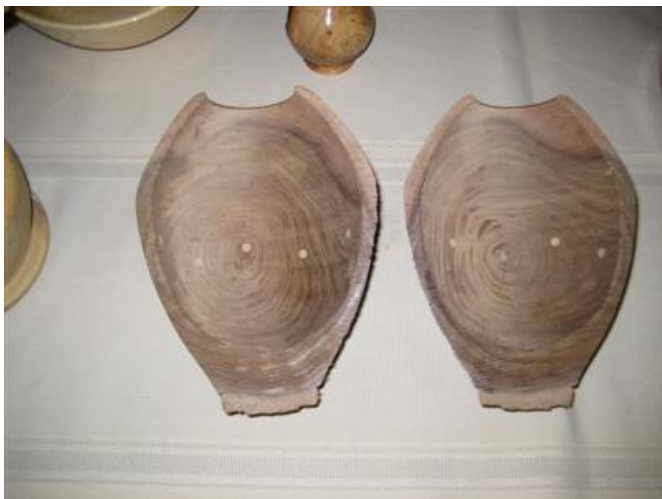
He also had a hollowform, which had developed a crack, so he cut it in two so that we could see how it was hollowed.
