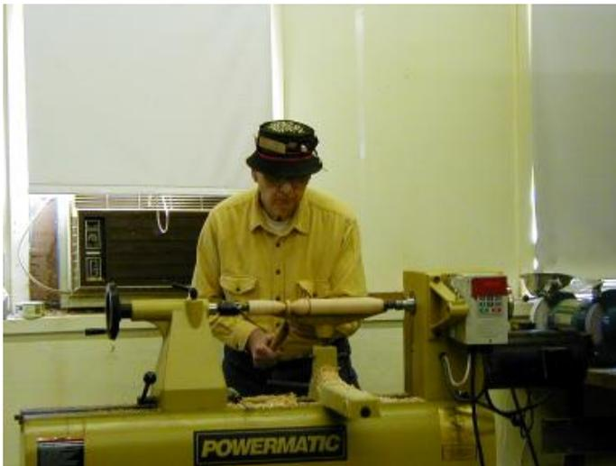
**He demonstrated how to turn a captured ring (using a skew).**
